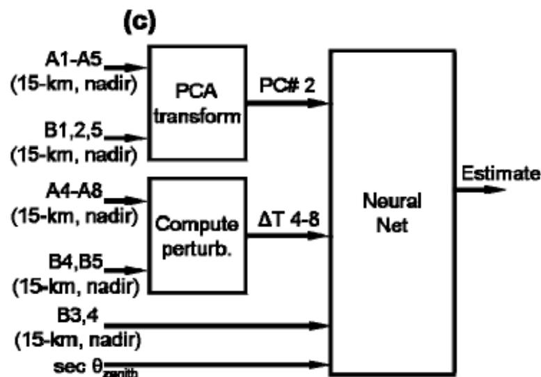
All neural networks have three layers with 10, 5, and 1 neuron, respectively, where the first two layers employ tangent sigmoid operators, and the final layer is linear.
