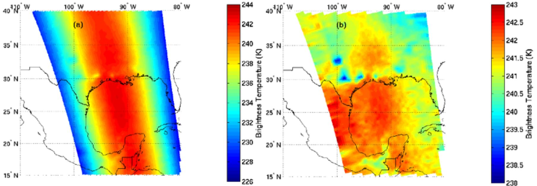
**NOAA-15 AMSU-A 54.4-GHz brightness temperatures for a northbound track on 13 Sept 2000. (a) Uncorrected, and (b) Limb-and-surface corrected**
