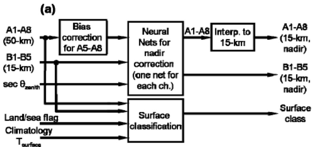
(a) Architecture for surface classification and for estimation of brightness temperatures that would have been seen at nadir.
