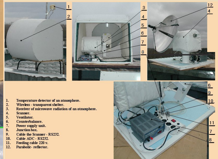
Fig. 1. A general view meteorological temperature profilers MTP5_5.pl.
