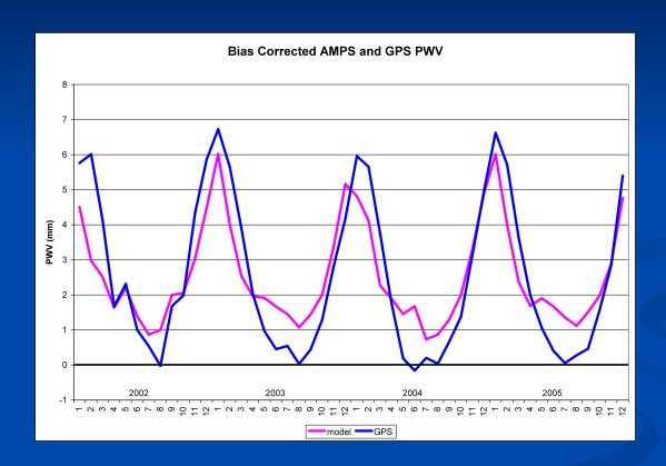
Removing the long-term average bias (2.82) shows that the GPS observations have a larger annual cycle than AMPS, and occasional differences in phasing
