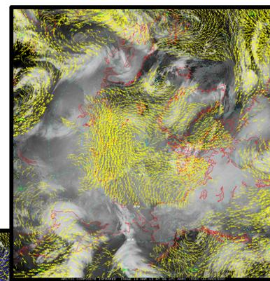
Atmospheric motion vectors (AMVs) from geostationary and polar orbiting satellites do not cover a belt in the high latitudes. However, AMVs from a version of the composites does as depicted in this display 6 hours coverage of AMVs from 19 March 2013 from 3 to 9 UTC.
