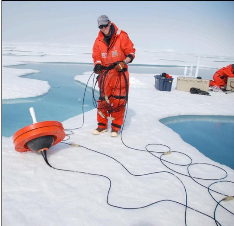
Preparing the thermistor string for playing through a hole augered into the ice.
