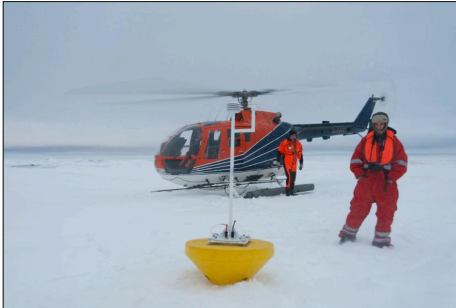
Ice Beacon deployed via helicopter and a sling by the crew of the Polarstern in the Arctic.
