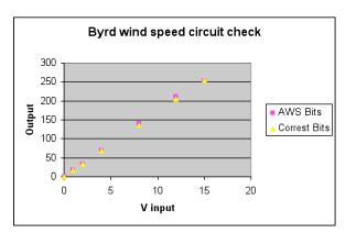
The overall accuracy of the wind speed circuit was within 2% after 30 years.
