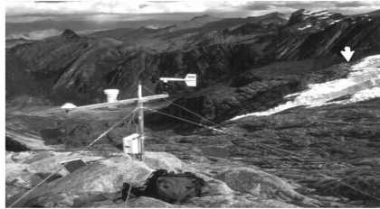
Figure 2. The automatic weather station (AWS) on a side ridge of Glacier Kurichinchey (Cordillera Blanca, Peru) in the approximate altitude of the equilibrium line (Rurichinchey EL). The horizontal support carries the sensors (from left to right): incoming shortwave radiation, temperature/humidity and wind. The background documents the overall environment of the study site. The glacier tongue of Glacier Rurichinchey is shown on the right side, the arrow labels the position of the glacier forefield AWS (Rurichinchey FF), which actually stands slightly behind the ridge. See color version of this figure at back of this issue.
