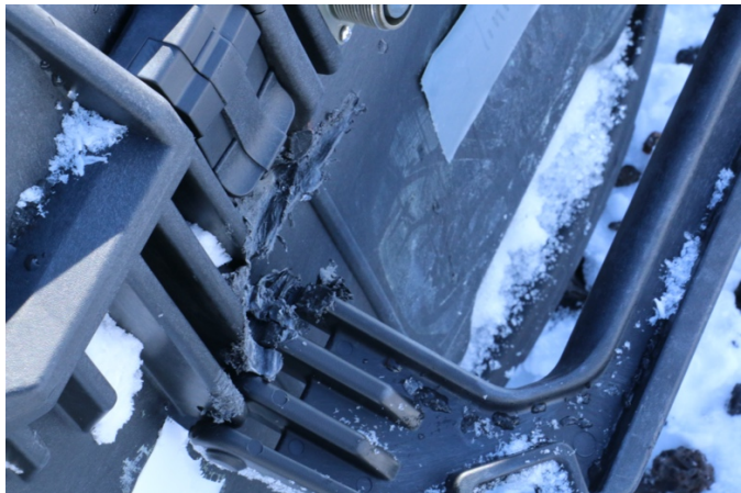
Damage to old power system case
