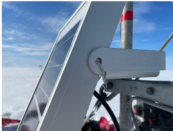
Wire used to attach solar panel to mount on SRH
