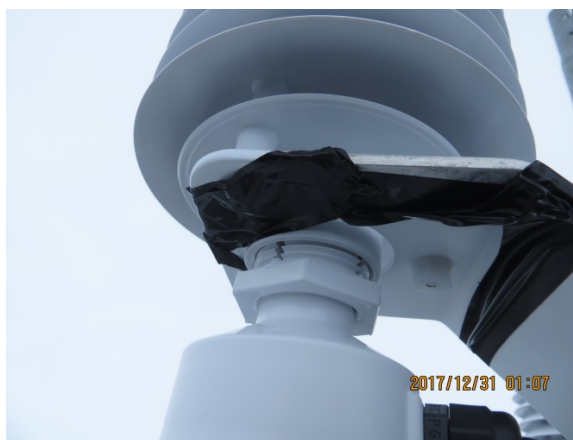
The tape job for the rod without a nut
