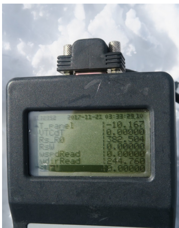
MNB wind direction 244.760° and wind speed of 0 m/s
