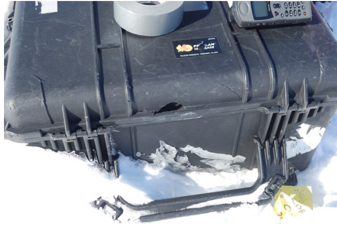
Lorne Electronics with new modem and battery box showing damage to the side seam.
