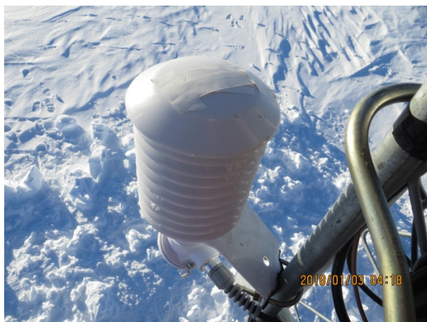
The repairs to lower temp Gill shield
