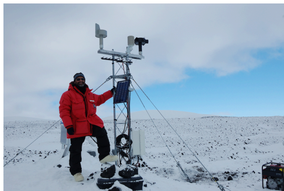
Finished installation of new guys and temperature sensor
