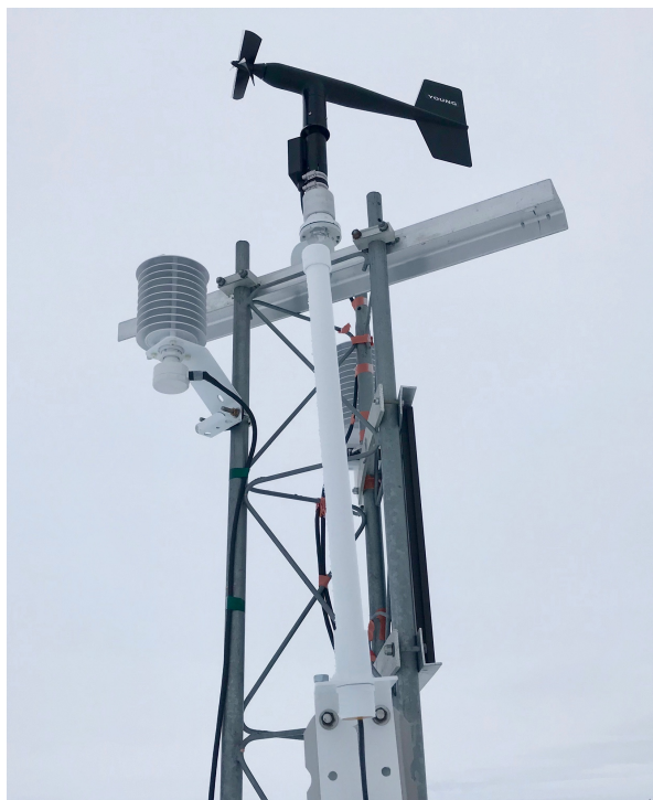
D-10 new upper temperature sensor
