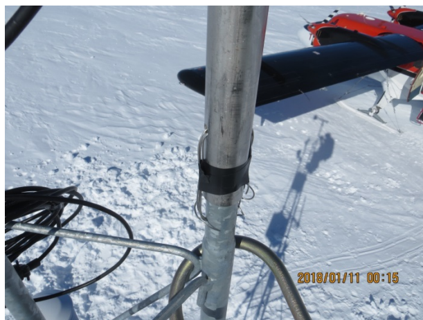
The anemometer pipe mounting.
