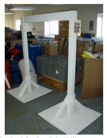
Figure 2. Mounting platform for radiation shield/temperature sensor testing.
