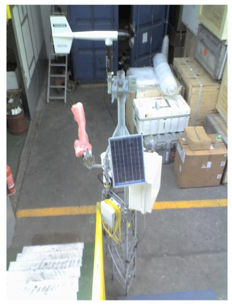
Image A32: AWS for Hugo Island under test in Punta Arenas
