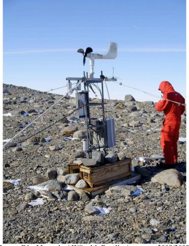
Image B1: Manuela AWS with Bendix Aerovane 2008/2009
