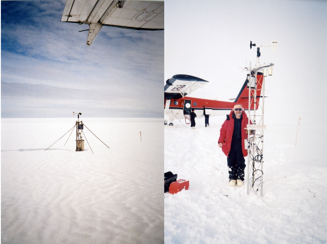
Figure A4. Swithinbank AWS before and after raising the tower.
