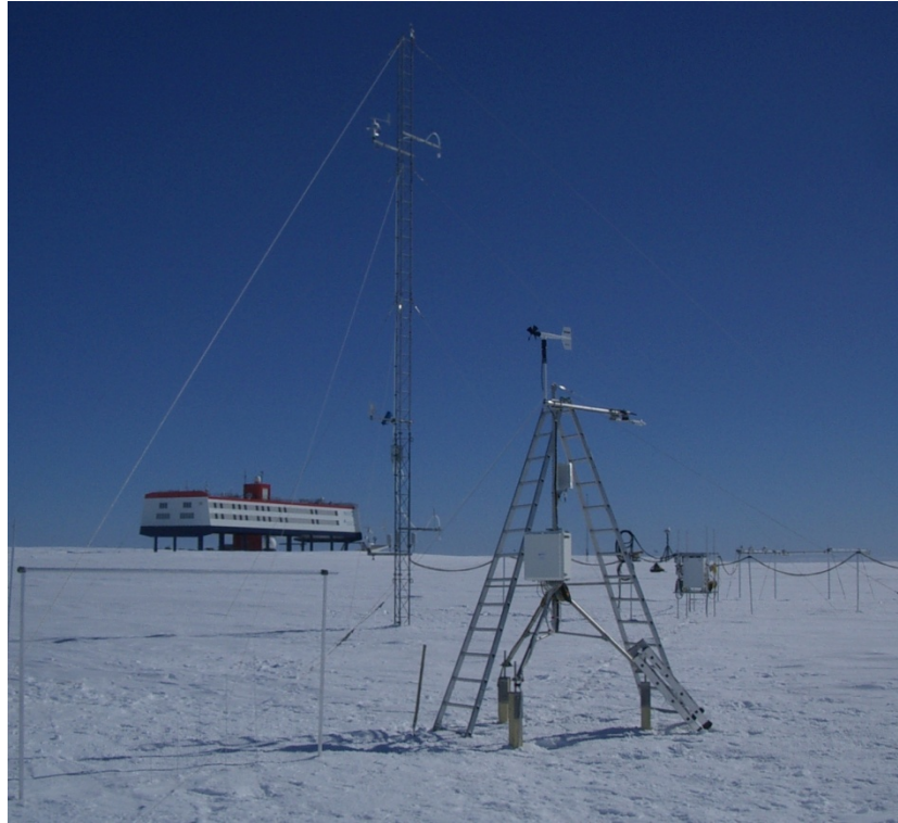
Installation of an AWS close to the meteorological instruments of Neumayer
